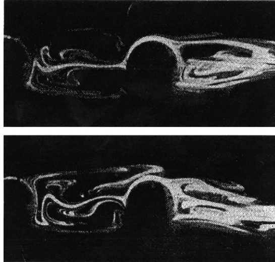
Fig. 7. Gap flow patterns for two tandem circular cylinders at intermediate pitch ratios ( L/D = 3 ) at Re = 100 , representative of the extended-body regime, flow from left to right.
